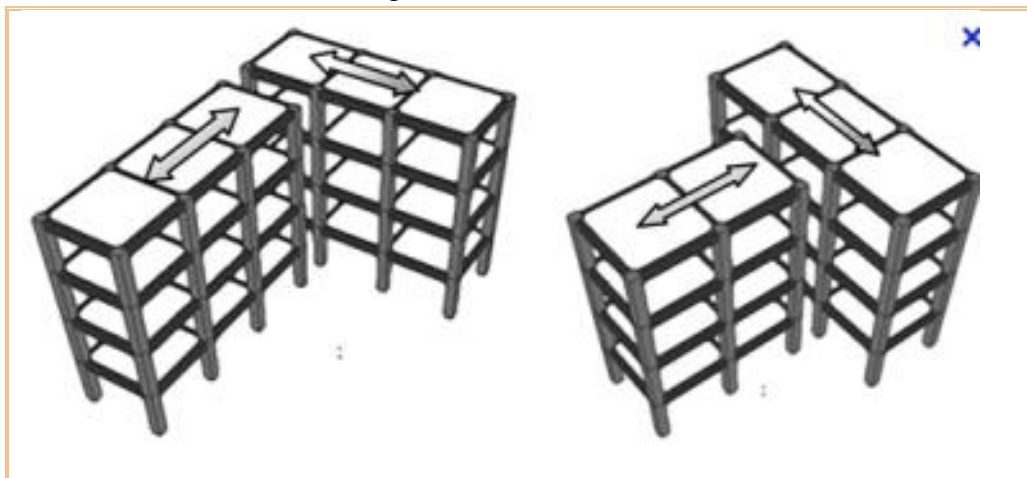
Fig(27) dividing building into simpler shape to avoid re-entrant corner (Korkmaz, 2011)
