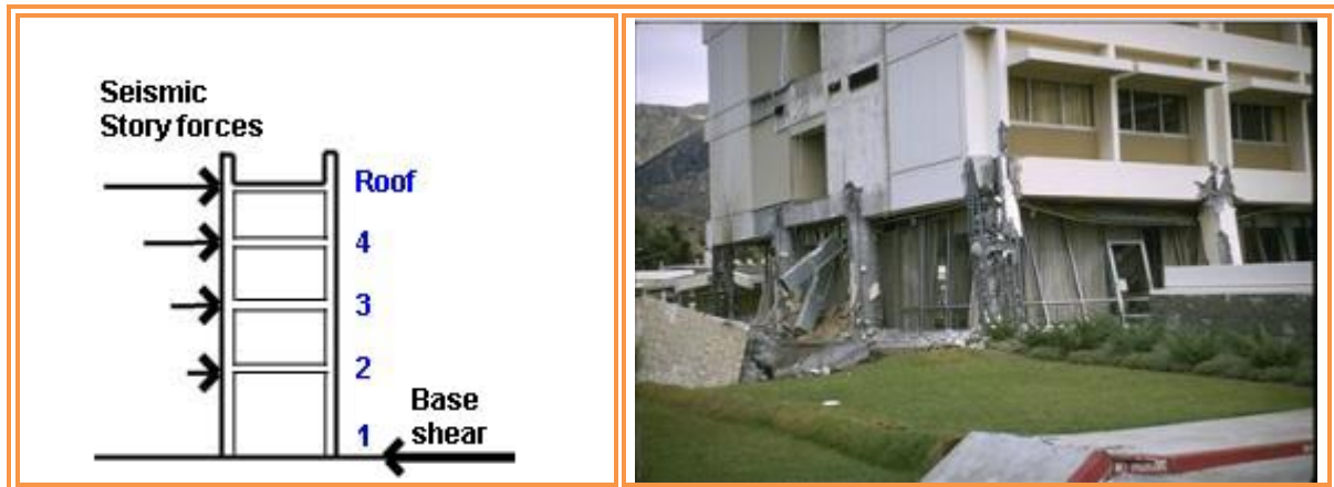
Fig (4) base shear mechanism and effects on the building (Ochshorn, 2009)
